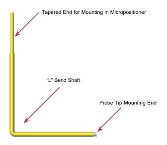
This "L" configuration is used when platen–positioner is well above the wafer-sample (Available with Delrin, Teflon,& Ceramic-Coax Shielding) Typical Use: Special-purpose wafer probing when probe mount is well above the wafer chuck- recommended use with Pivot head style micropositioner.
