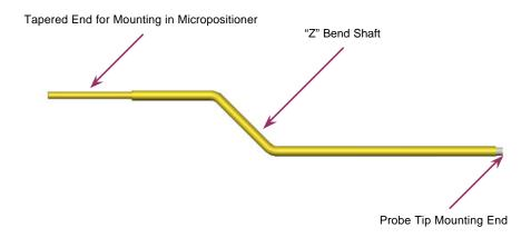
This "Z" configuration is used to drop the tip down to the bottom of the platen surface, just above the wafer-sample (Available with Delrin, Teflon, & Ceramic-Coax Shielding)
