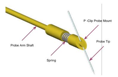
The "P"-style probe holder accepts all the Signatone manufactured probe needles.
