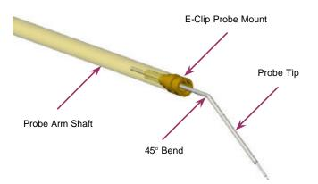
The "E"-style probe holder accepts probe needles with 0.015 – 0.020 diameter wire. (Available with Delrin & Teflon-Coax Shielding) Typical Use: Areas with small working distance & package devices
