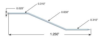
The SE-T may be used with the "S" & "P" Signatone probe tip holders. Typical Use: Probing pads and geometries  $10\mu$ >
