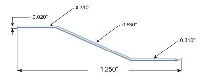
The SE-20TZ may be use is any of the Signatone probe tip holders. Typical Use: Probing pads and geometries  $5\mu$ >
