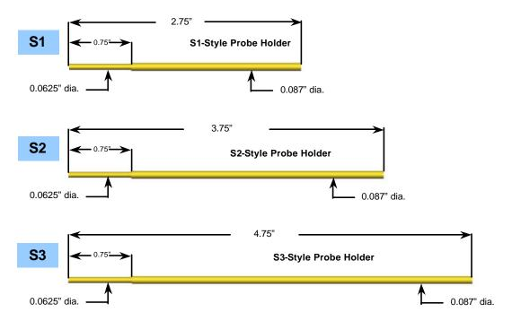
All three versions (S1, S2,& S3) includes 0.075" taper for mounting into all styles & vintage of Signatone micropositioners (Available with Delrin, Teflon, & Ceramic-Coax Shielding)
