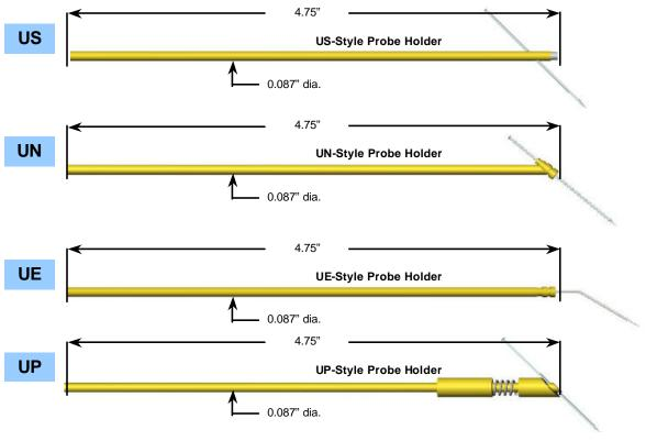
(Available with Delrin, Teflon, & Ceramic-Coax Shielding)
