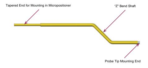
This "Z" configuration is used w/ a probe card to drop the tip down over the probe card adapter, just above the wafer-sample (Available with Delrin, Teflon, & Ceramic-Coax Shielding) Typical Use: General-purpose wafer probing w/ probe cardsrecommended use with Pivot head style micropositioner.
