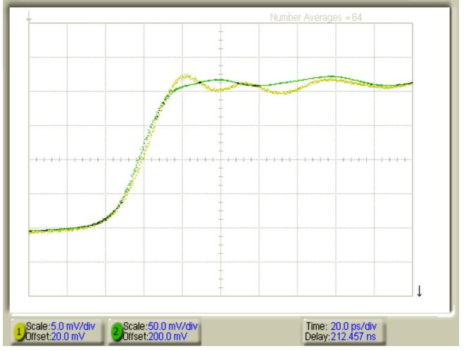
This plot shows the response of the Model 35 Picoprobe to a 0.25 volt, 25 picosecond rise time input pulse. Both the input pulse(Channel 2) and the Model 35 response (Channel 1) are displayed simultaneously on a dual channel 20 GHz sampling oscilloscope. The Model 35 probe tip was contacted to a 50 ohm impedance strip line that carried the input signal. The Model 35 used only a single contact and did not require a short ground connection.
